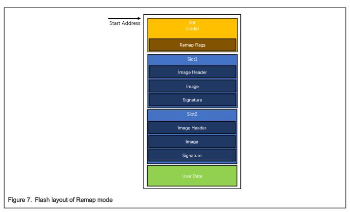
Similar to the division of Swap mode, it is divided into SBL, Slot1, Slot2, and User Data. The difference is that the Image Trailer part of the flag that stores the FOTA process in Slot1 and Slot2 has been canceled. Instead, at the end of the SBL region, set a structure called Remap Flags to control the FOTA process.
