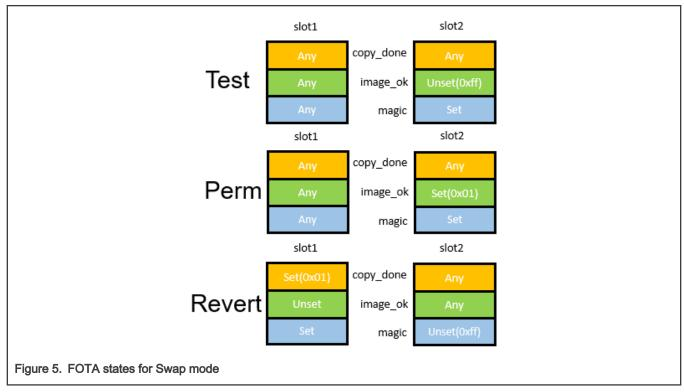
All Image Trailer values that do not belong to the above three states are None state, and no image exchange occur. In the actual SBL project, the image revert function is supported by default, so the Perm state is not used.
