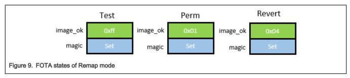
The Revert function of Remap mode is implemented based on the value of the <code>image\_ok</code> field. When SFW receives a new image, it reads the <code>image\_position</code> field in Remap Flags, gets the slot where the current firmware is located, stores the new firmware image in another slot, and writes the magic value to the corresponding field of Remap Flags. After rebooting back to SBL, SBL reads the location of the current firmware image and gets to the Test state.
