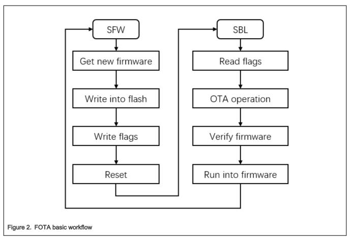
Many i.MXRT series MCUs chips have the remap function, so SBL and SFW define two different modes on FOTA: Swap mode and Remap mode. The operations corresponding to the write flags, read flags, and OTA operation in the flowchart are different, as described in Swap mode and Remap mode.
