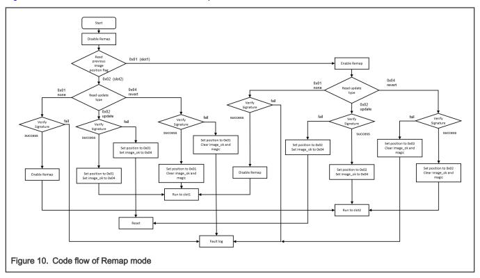
During the whole judgment process, when the signature of the updated firmware fails to pass the verification, SBL actively restarts the board, re-enters the judgment process of SBL, gets the revert state, and completes the program rollback.
