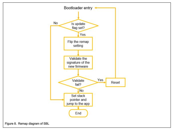
Since the entire Slot has been remapped and the content of the flag has changed, the Remap Flags cannot be set in Slot1 and Slot2. The SBL and SFW projects use the last 32 bytes of the SBL area in the flash as Remap Flags. The revert of firmware images is also supported in Remap mode. The state of Remap Flags controls the FOTA process. In remap mode in SBL, FOTA defines four states, Test, Perm, Revert, and None.
