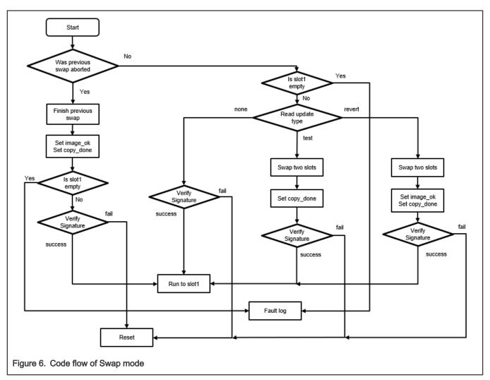
The exchange of two Slots in the Swap mode does not use the third flash piece. The size of the firmware image cannot exceed the size of the Slot minus the size of the two Sectors (one is the Image Trailer part). SBL uses the method below to finish the exchange. For image in Slot1, shift the entire firmware to the lower address by one sector size, copy the first sector of Slot2 to the first Sector of Slot1, copy the second sector of Slot1 to the first sector of Slot1, and so on.
