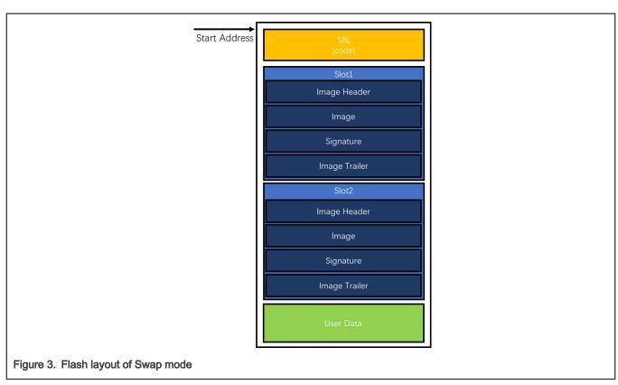
SBL is at the start of the flash. The ROM of the i.MXRT series chips jumps to this position in XIP mode. The firmware images stored in Slot1 and Slot2 are composed of four parts. Image Header is at the top of the image. It tores the length, version number, and other information of the firmware. Following the Image Header is the firmware itself. The firmware signature is behind the Image. At the end of the slots is the Image Trailer, which stores the flag of the FOTA process.
