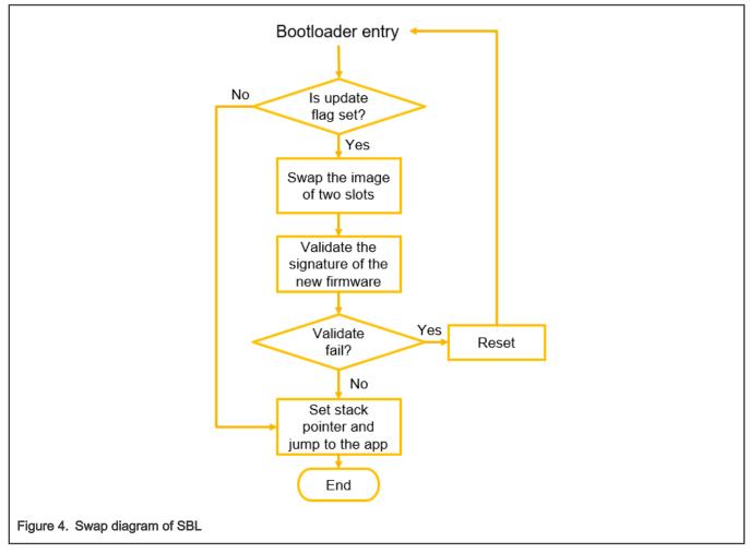
Figure 4 shows the basic logic of the Swap mode in SBL. SFW resets the MCU, the code runs into SBL, and the process of the SBL is slightly different from the process in mcuboot. In the mcuboot project, first verify the signature of the new image stored in
