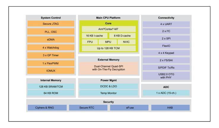
View additional information for i.MX RT1010 Crossover MCU with Arm® Cortex®-M7 Core Operating Up to 500 MHz.
